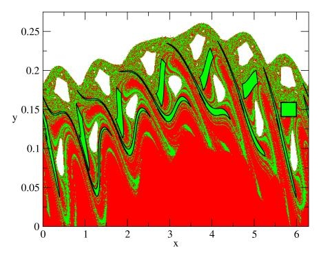
Fig. 4. Backward iterates of the rectangular box for which exit basins of field lines are painted green. The exit basin of the tokamak wall is painted red. Parameters are the same as in the previous figure.
