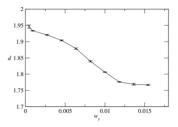
Fig. 8. Uncertainty dimension for the boundaries of the exit basins as a function of the exit width. Orbits escape either through the tokamak wall (y = 0) and a rectangular box centered at (x = 3.1, y = 0.22) and widths  $w_y$  and  $w_x = 20w_y$ .
