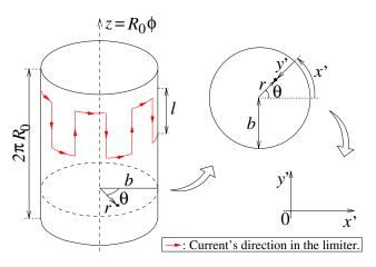
Fig. 1. Schematic view of the tokamak in the periodic cylinder approximation, its Poincaré section, and the rectangular coordinates (before normalization) used to describe magnetic field lines.
