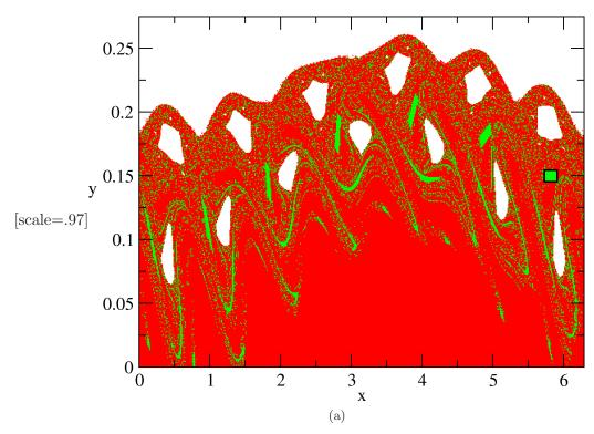
Fig. 3. Exit basins for orbits escaping through the tokamak wall (red) at y = 0, and through an exit (green) with width (a)  $w_y = 0.0045$  and (b)  $w_y = 0.0090$ , with  $w_x = 20w_y$ . White regions are for orbits which never escape through either exit region. The limiter perturbation has m = 7 and  $I_h/I_p = 0.06$ .
