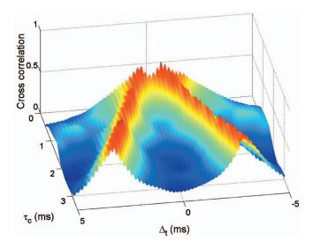
FIG. 2. (Color) Cross-correlation plot of Chua circuits A and B, as a function of the time shift  $\Delta t$  between both series and the time delay  $\tau_c$ . We can observe how the highest correlation ( $C_{\rm max} \sim 0.64$ ) always occurs at  $\Delta t = \pm \tau_c$ , which indicates that we have lag synchronization with exchanges in the leader-follower roles between both circuits.
