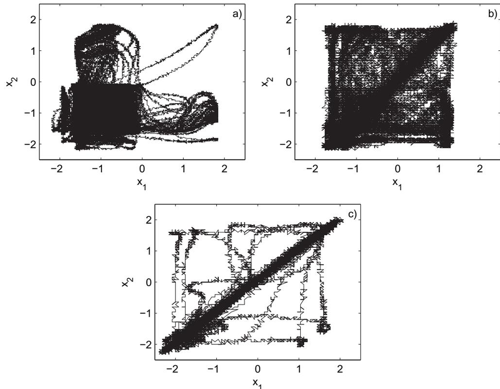
**Figure 12.** Experimental  $(x_1, x_2)$  diagrams for both neurons in (a) the noiseless case, (b) white noise ( $R \approx 0.6$ ) and (c) coloured noise ( $R \approx 0.9$ ). In the noiseless case, the neurons are not synchronized at all. The synchronization improves when noise is added to the FHN systems, but it is far from being perfect.
