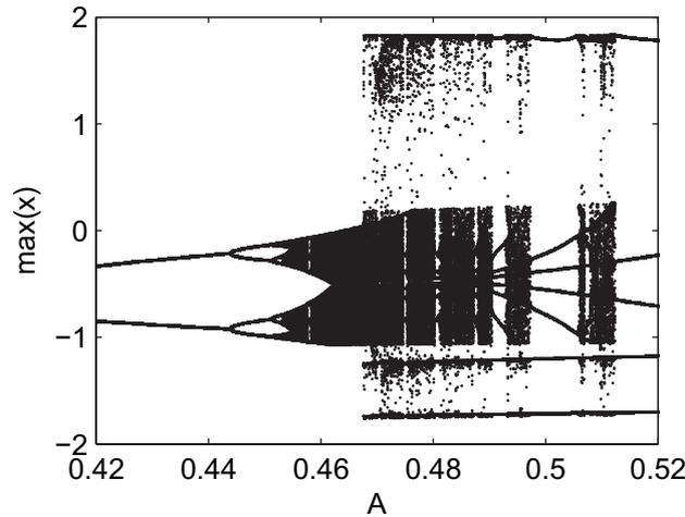
**Figure 1.** Numerical bifurcation diagram for the voltage variable  $x$  by taking as control parameter the amplitude of the external forcing  $A$ . The spiking regime is observed for high values of  $A$ , whereas the non-spiking regime is observed for low values of  $A$ . Parameter values are  $a = 0.7$ ,  $b = 0.8$ ,  $c = 12.5$  and  $T = 0.636$ .
