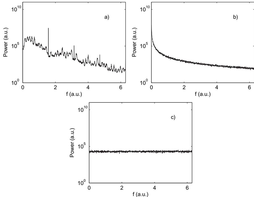
**Figure 3.** Plots of (a) the power spectrum of the noiseless forced FHN; the main peak is observed at the forcing frequency  $1/T$ ; (b) the power spectrum of the coloured noise whose  $\gamma$  matches the half-width of the spectrum of the noiseless forced FHN; and (c) the power spectrum of white noise. Both spectra ((b) and (c)) correspond to noise with the same  $\sigma$ .
