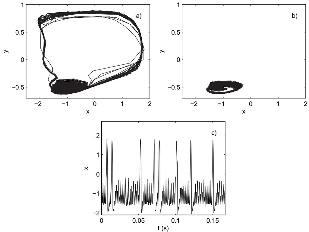
**Figure 2.** Experimental trajectories in the phase space corresponding to (a) the spiking regime, (b) the non-spiking regime and (c) the time sequence from which (a) is extracted. One can see that the low amplitude between large spikes is mainly a forced limit cycle and is perturbed by the chaotic dynamics.
