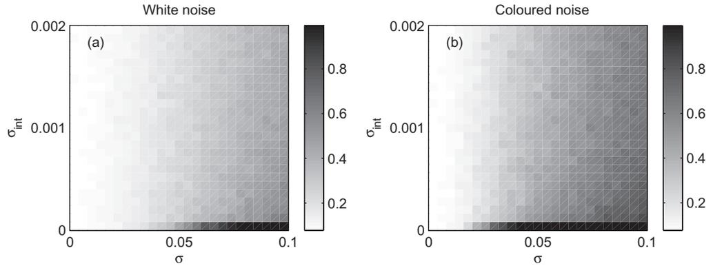
**Figure 10.** Synchronization rate as a function of (a) the common noise and (b) the intrinsic noise. Darker colours indicate higher values of the synchronization rate. Notice, for both white and coloured noise, the strong influence of the intrinsic noise, which causes an important decrease in the synchronization rate. We obtain the best performance for  $\sigma_{\text{int}} = 0$  and large values of the common noise  $\sigma$ .
