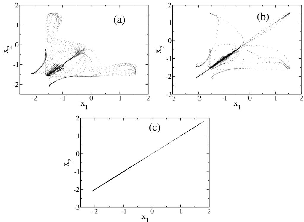
**Figure 4.** Effect of white noise in the synchronization phenomenon between the two FHN systems. Parameter values are as follows:  $A = 0.471$ ,  $a = 0.7$  and  $T = 0.636$  and (a)  $\sigma = 0$ , (b)  $\sigma = 0.01$  and (c)  $\sigma = 0.05$ . The intensity of noise plays a crucial role in the synchronization.
