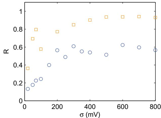
**Figure 13.** The synchronization rate  $R$  (see text for details) versus the standard deviation of noise  $\sigma$  obtained in the experiments for white noise ((blue)  $\circ$ ) and coloured noise ((orange)  $\square$ ). In both cases, the noise produces a positive effect on the synchronization between the two neurons, which is better for coloured noise.
