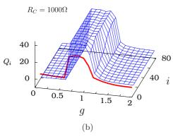
Fig. 9.  $Q_i$  as a function of i and g for two values of  $R_C$  illustrating (a) damped propagation of signal (for  $R_C=2.165~\mathrm{k}\Omega$ ) and (b) undamped signal propagation (for  $R_C=1~\mathrm{k}\Omega$ ) through the unidirectionally coupled Chua's circuits. The thick red curve in (b) represents  $Q_1$ . In (a)  $Q_1$  is not shown because  $Q_i$ 's with i>1 are much lower than  $Q_1$ .
