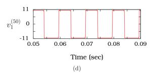
Fig. 11. Evolution of  $v_1^{(i)}$  with time at four different nodes denoted as i where  $R=2.15\,\mathrm{k}\Omega,\,R_C=1\,\mathrm{k}\Omega$  and  $g=1.1\,\mathrm{V}.$  Notice the suppression of high-frequency oscillations as i increases. (a) i=1, (b) i=5, (c) i=15 and (d) i=50.
