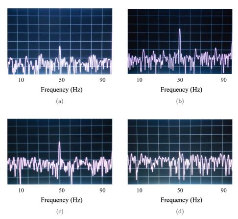
Fig. 2. The power spectrum of the voltage  $v_1$  for four values of g. (a) g=1 V, (b) g=1.3 V, (c) g=1.55 V and (d) g=2 V. The values of other circuit parameters are  $C_1=10\,\mathrm{nF},~C_2=100\,\mathrm{nF},~L=18\,\mathrm{mH},~R=1.98\,\mathrm{k}\Omega,~A=0.3$  V,  $\omega=50$  Hz and  $\Omega=500$  Hz.
