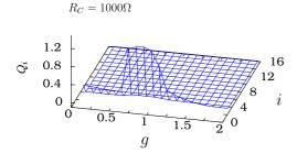
Fig. 12.  $Q_i$  as a function of g and i for  $R_C = 1000 \Omega$ . For clarity  $Q_1$  is not shown because  $Q_1(g)$  is  $\gg Q_i$  for  $i = 2, 3, \ldots$
