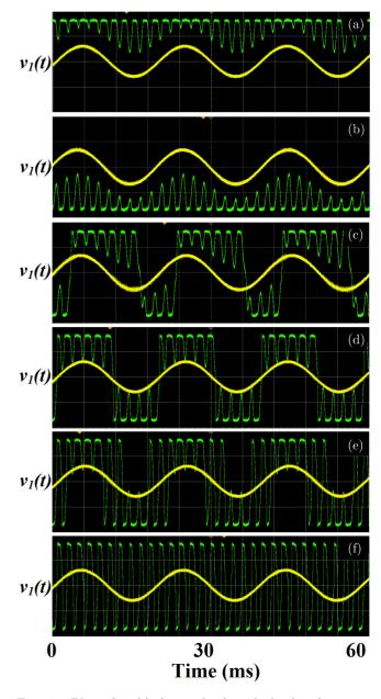
Fig. 4. Plot of  $v_1(t)$  (green line) and the low-frequency periodic input signal  $f \sin \omega t$  (yellow line) versus time t for five values of the amplitude g of the high-frequency periodic signal. (a) and (b) g=1V, (c) g=1.15V, (d) g=1.3V, (e) g=1.55V and (f) g=2V. In all the subplots the range of  $v_1(t)$  is [-10V, 10V]. The low-frequency periodic input is 10 times enlarged in all the subplots for clarity.
