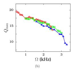
Fig. 6. Plot of (a)  $g_{\rm VR}$ , the critical value of g at which resonance occurs and (b)  $Q_{\rm max}$ , the value of Q at  $g=g_{\rm VR}$  versus the high-frequency  $\Omega$  of the driving force. The values of the parameters are  $f=0.3\,{\rm V}$  and  $\omega=50\,{\rm Hz}$  (for the symbol circle),  $\omega=100\,{\rm Hz}$  (square) and  $\omega=150\,{\rm Hz}$  (triangle).
