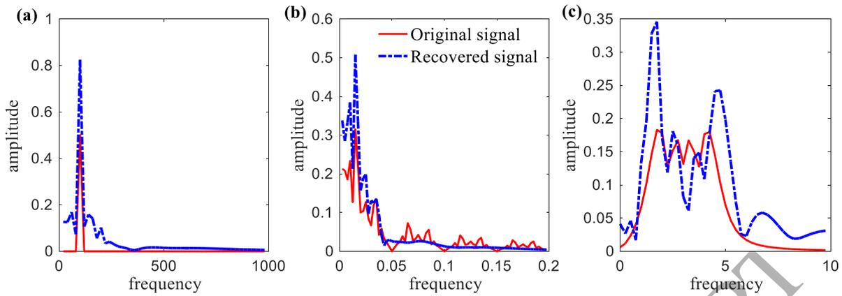
Fig. 10. The frequency spectrums of the recovered signals and original signals. (a) Harmonic signal, (b) binary signal, (c) chirp signal.
