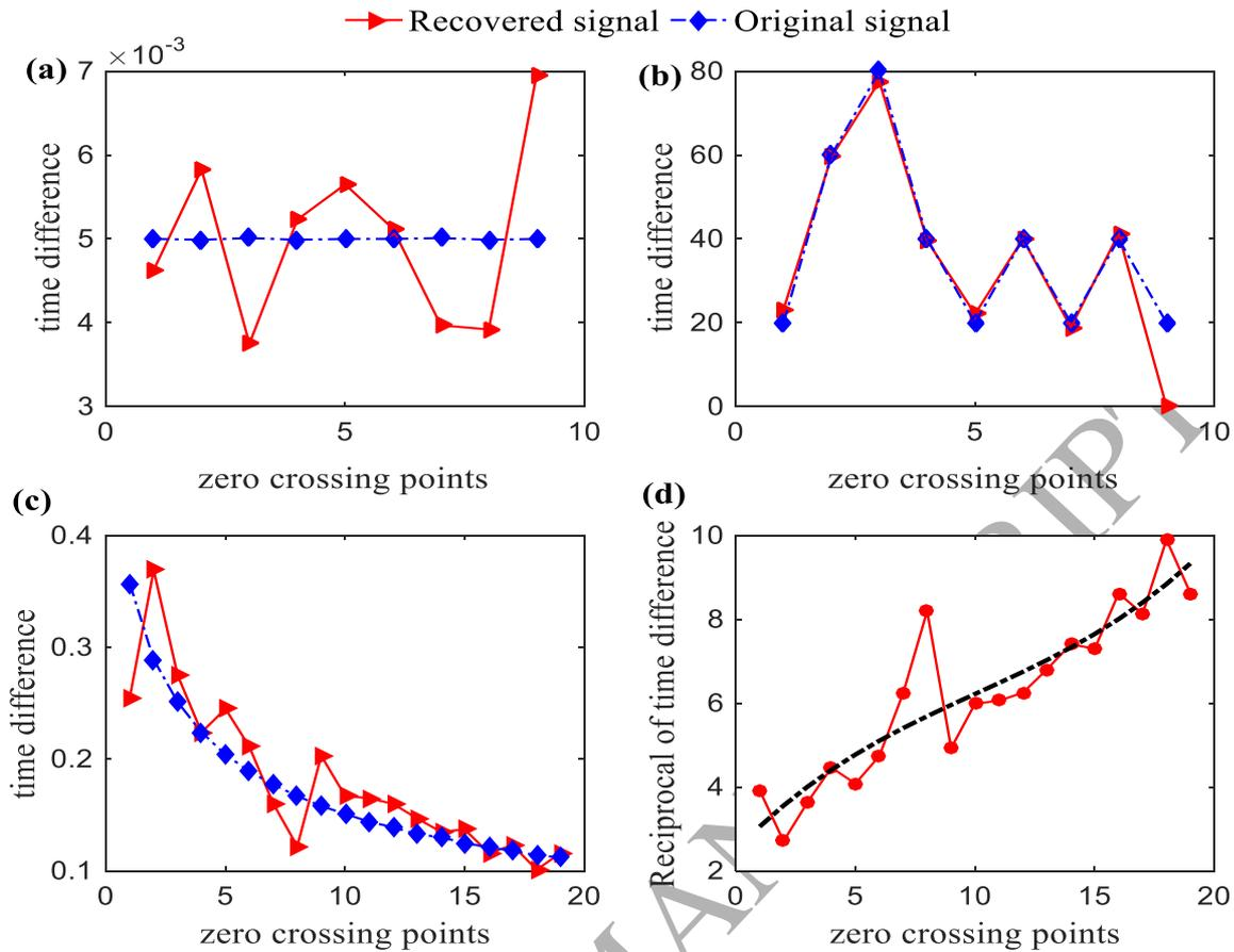
Fig. 9. The value of time difference depends on the zero crossing point. (a) Harmonic signal, (b) binary signal, (c) chirp signal, (d) The reciprocals of time difference values shown in subfigure (c).
