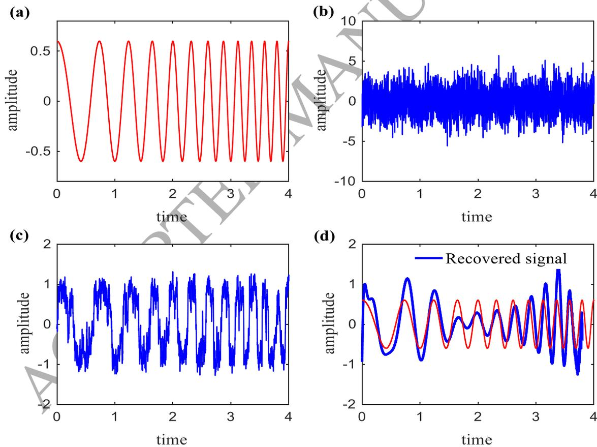
Fig. 8. The recovery of a chirp signal. (a) The raw chirp signal, (b) the chirp signal contaminated by a strong Gaussian white noise, (c) the output of the nonlinear system follows the original input signal under the minimum PMV criterion, (d) the recovered signal attained by the polynomial fitting on the basis of subfigure (c).
