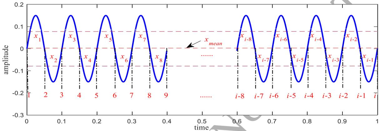
Fig.3. The realization of PMV indicator by using the harmonic signal as an example.
