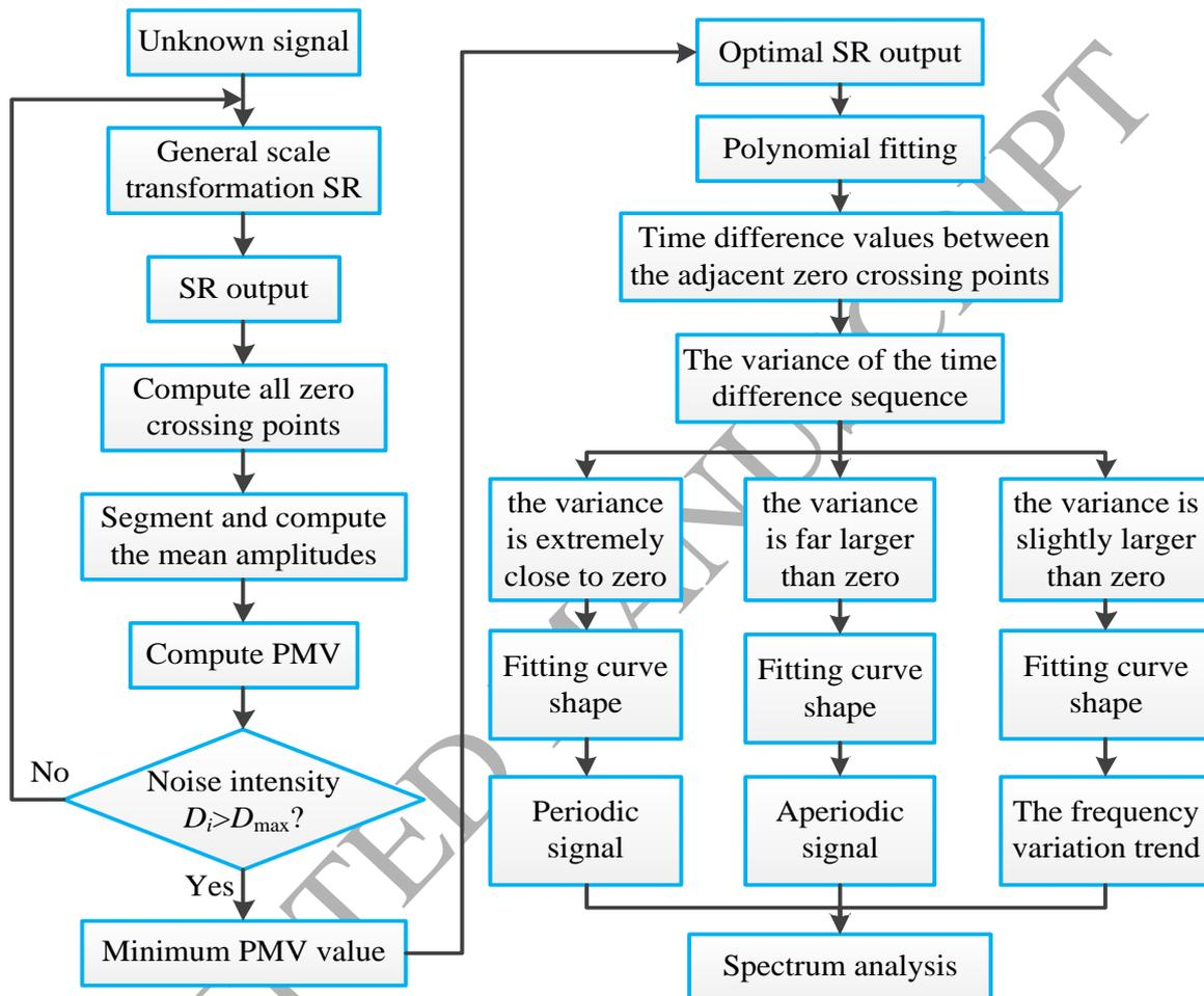
Fig. 4. The flowchart of realizing the PMV indicator and the parameters estimation strategy.
