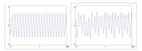
Fig. 4. Evolution of velocity over time for periodic and chaotic motions.
